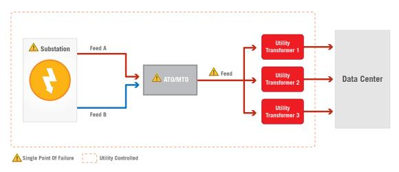
Only one power feed at a time is passed from the ATO to the transformers.
